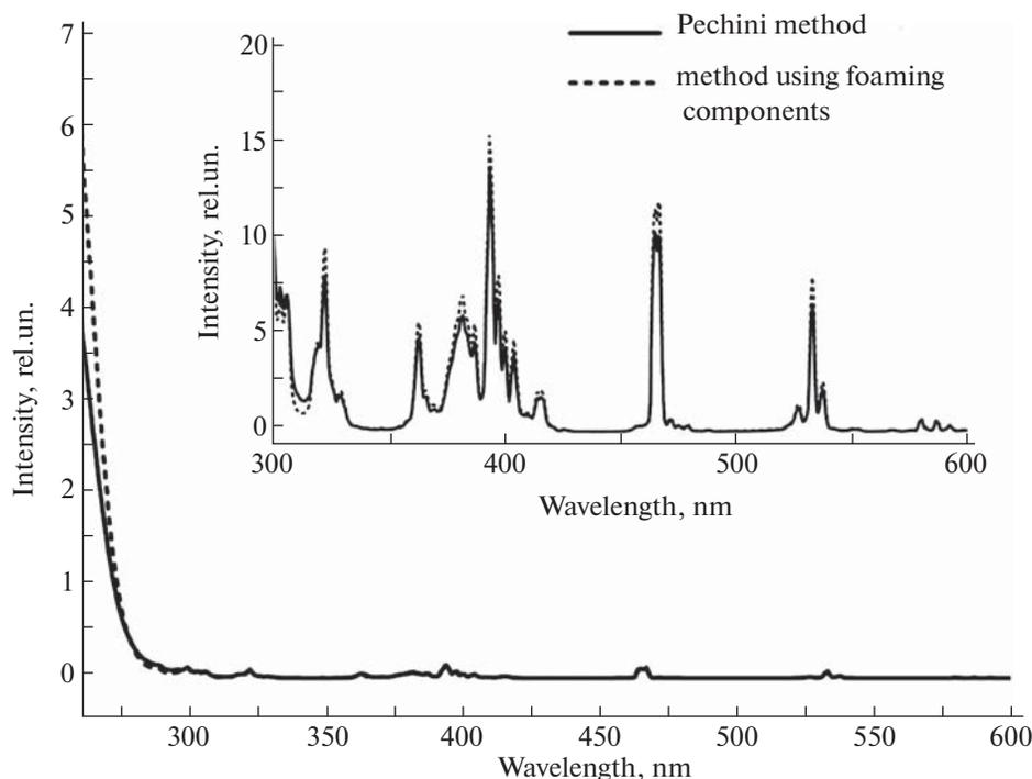
**Fig. 6.** Luminescence excitation spectra of the samples of  $\text{Y}_2\text{O}_3:\text{Eu}^{3+}$  synthesized via the Pechini method and the method using foaming components ( $\lambda_{\text{lum}} = 610.2$  nm).
