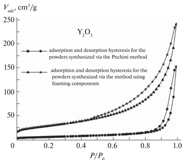
**Fig. 2.** Adsorption and desorption isotherms for the powders synthesized via the standard Pechini method and a method using foaming components.
