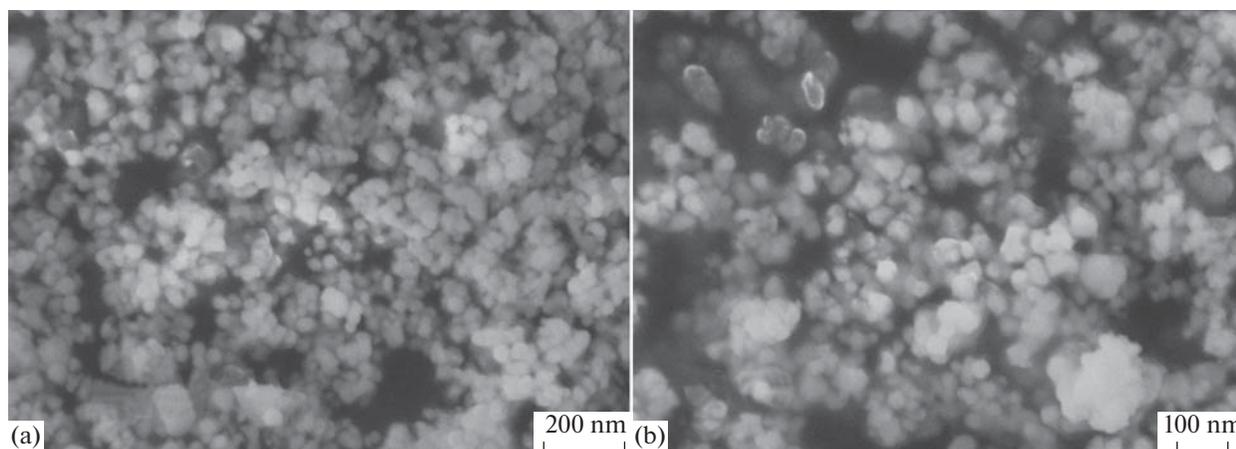
**Fig. 4.** Micrographs of the samples of  $Y_2O_3$  synthesized via the method using foaming components at 1000°C, 2 h.
