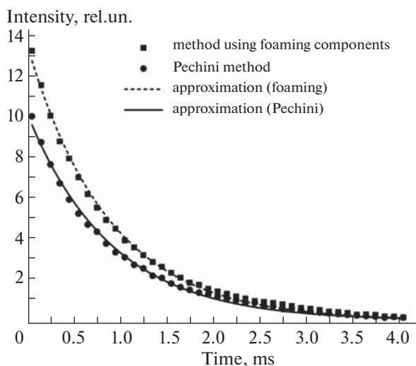
**Fig. 7.** Kinetics of the luminescence of the samples of  $Y_2O_3:Eu^{3+}$  synthesized via the Pechini method and the method using foaming components ( $\lambda_{exc} = 393.5$  nm and  $\lambda_{lum} = 610.2$  nm).
