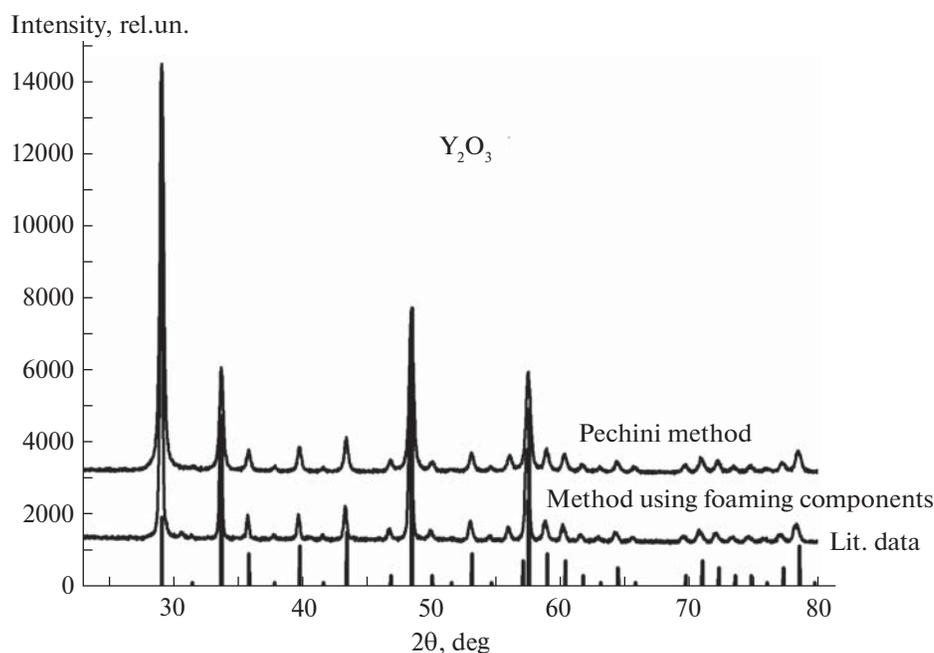
**Fig. 1.** Diffraction patterns of the samples of Y<sub>2</sub>O<sub>3</sub> synthesized via the Pechini method and a method using foaming components under similar temperature and time modes (900°C, 2 h).
