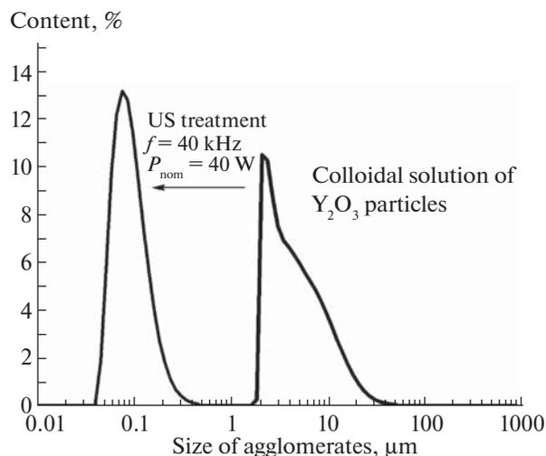
**Fig. 3.** Particle-size distribution of yttrium oxide before and after US treatment. Synthesis via the method using foaming components.
