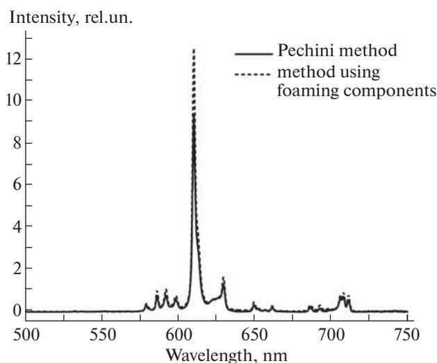
**Fig. 5.** Luminescence spectra of the samples of  $\text{Y}_2\text{O}_3:\text{Eu}^{3+}$  synthesized via the Pechini method and the method using foaming components ( $\lambda_{\text{exc}} = 393.5$  nm).
